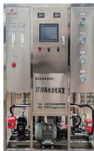
Seawater desalination equipment
